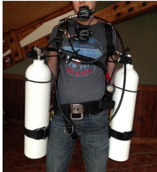
Pic. 13 Attaching the regulator – Right tank
